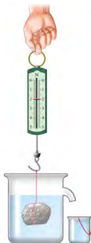
(b) 弹簧测力计的示数 F' = \underline{\quad} N, 物体所受浮力 F_{\text{浮}} = G - F' = \underline{\quad} N
