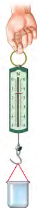
(c) 接水后杯子与水总重 G'_{\text{杯}} = \underline{\quad} N, 被物体排开水的重力 G_{\text{排}} = G'_{\text{杯}} - G_{\text{杯}} = \underline{\quad} N
